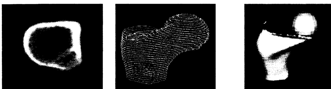
(a) Polyline contours used to demarcate boundary through the segmented images (b) Polyline grown through the segmented images (c) B-spline surfaces and primitives (sphere) used to model the femur anatomy
